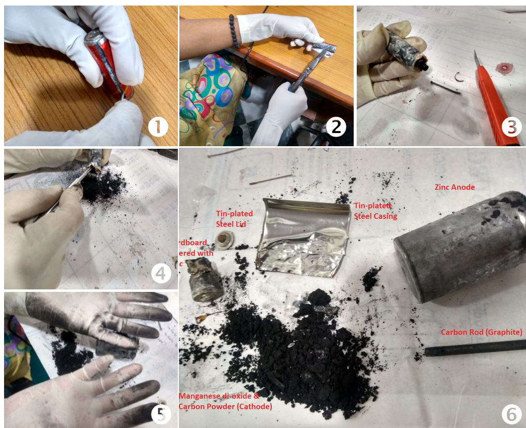
Figure 8: Stages of Battery Dismantling
